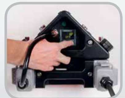
Setting temperature and pressure controller
